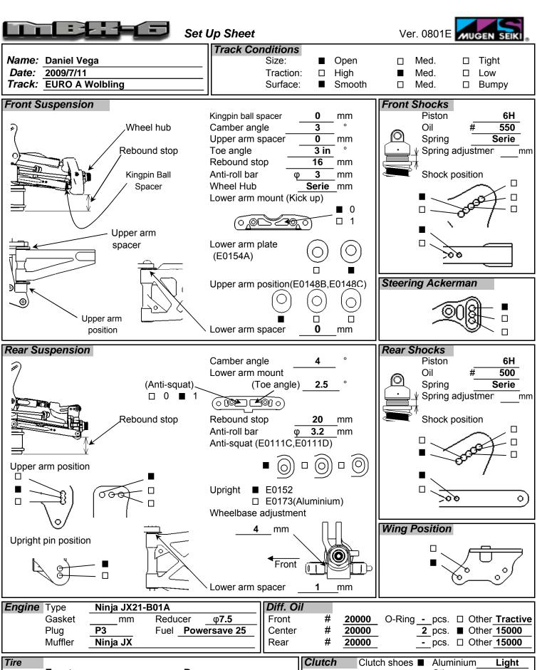
**Front** Rear □ Other Crosswobs vellow Type Type Crosswobs yellow Sprir 1.1 mm Foam Serie Foam Serie Clutch bell / Spur gear 13T / 46T Result Comments: The tractive diff from Fioroni used in front. The set up of the car is very good for long mains from 10 minutes to the end of the race.
